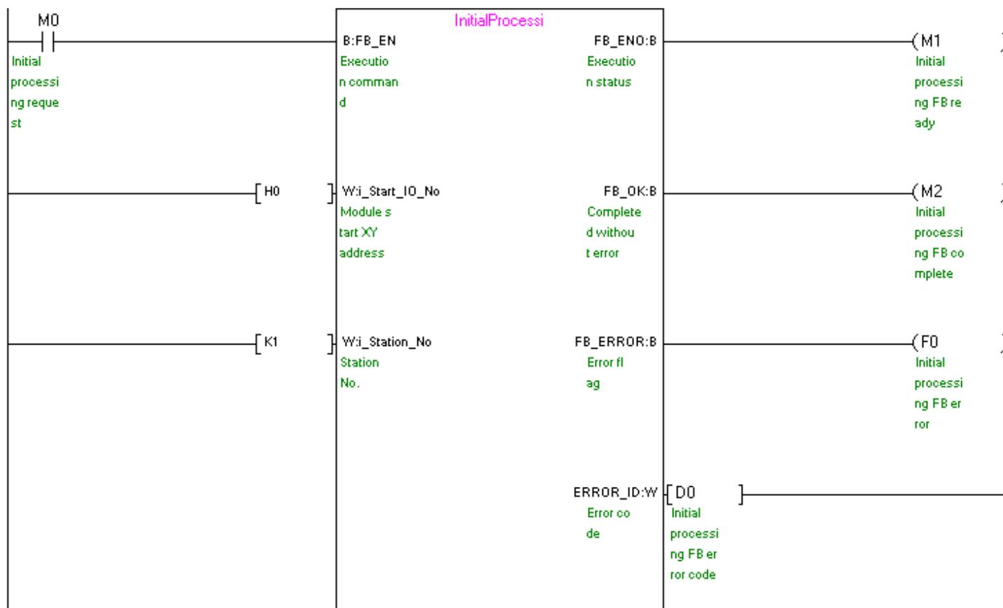
M+NZ2GF2B116\_SetOpeCondition (Operation condition setting)
